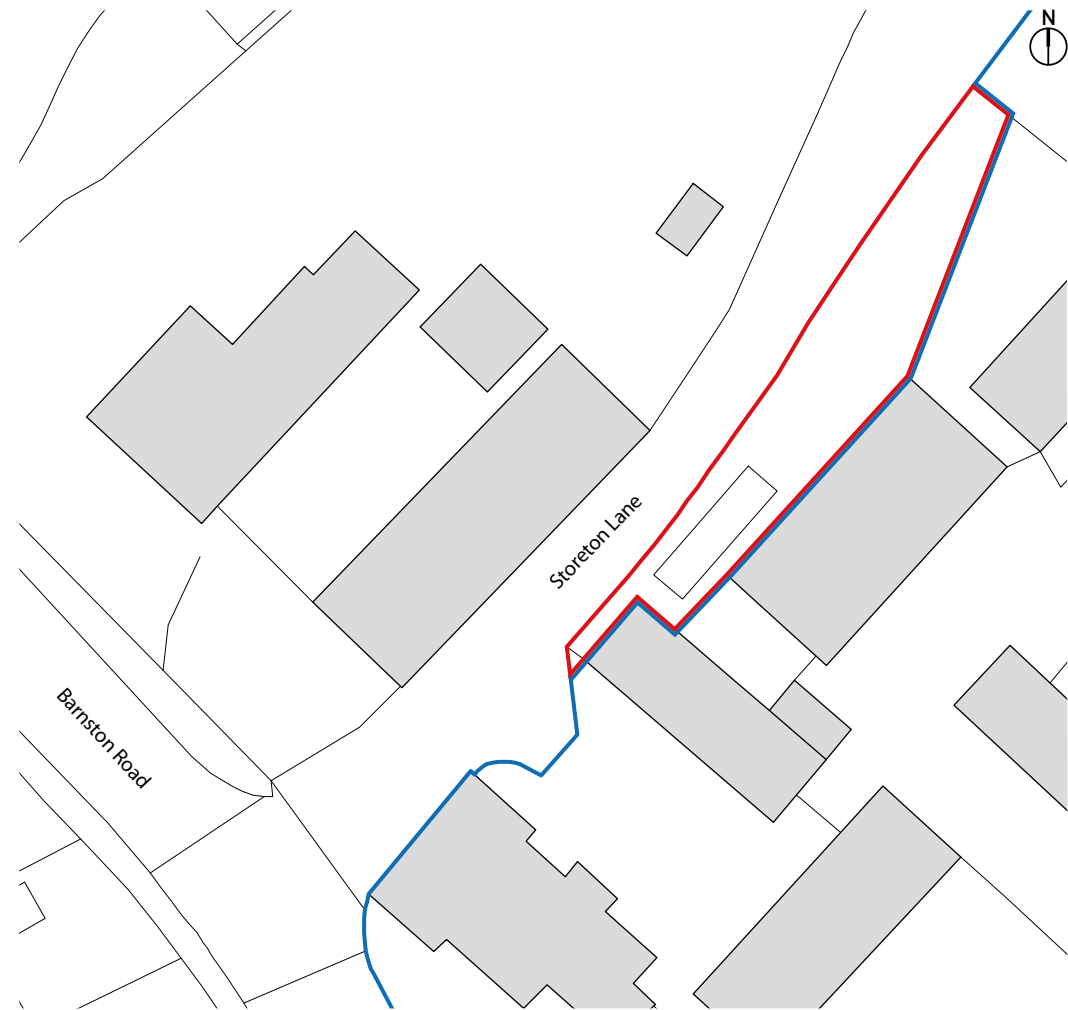
Figure 24: Storeton Lane widening location plan
